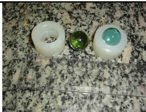
Figure 2. Image that shows in A) the holder; B) glass mold and C) assemblage to generate latex sheet with the technique proposed.
